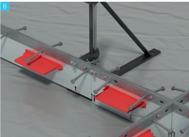
6 Continue to fit the ArmourJoints. Ensure the lapped joints are butted end to end tightly. Fit the plastic bolt and wing nut at the lapped joint.
