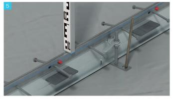
Connect as many Armour Joints together as required. Set the joints to the correct height by adjusting the flanged nuts on the feet. Tighten the nuts once the joint is at the correct height. Use a staff on the top faces of the joint and level (theodolite) to obtain the correct height. Small adjustments to height can be made once the concrete is poured as the joints may move slightly with the thrust of the concrete.
