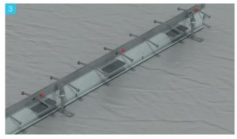
Once all of the feet are fitted, check the feet are orientated the correct way up, and the foot base plate with the pinning hole is on the side of the joint which will be the second side for casting.
