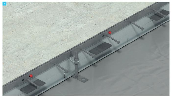
Once the first side of the joint has been cast with concrete and has cured, the second side (with the leave-in-place feet) can be cast. Remove the fixing pins which hold the feet in place and remove the intermediate bracing pins and wooden wedges. Shorten the threaded rod using an angle grinder if necessary. Cast concrete to the second side.
