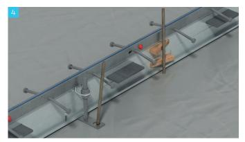
Place an Armour Joint (with feet fitted) under the string line and position it accurately. Drive road form pins through the hole in each of the feet base plate holes. Use additional fixing pins (dia 14 x 600mm long) and timber wedges to brace the joint between each foot.
