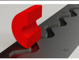
SHIELDJOINT is unique since it eliminates impact across the joint from Mechanical Handling Equipment (MHE) such as forklift trucks, but it also does not require any joint sealing. It's clever design ensures that no debris can enter in to the vertical gap between the two slabs. This design feature is useful in foodstuff warehouses where pest control is a paramount or food preparation areas (available in stainless steel).
